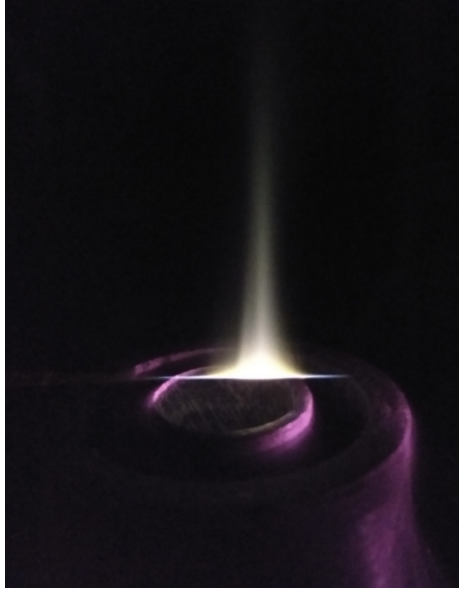
Figure 2.4: FLEET in free jet from co-flow nozzle. Note long-lived visible emission. Innermost diameter is 16 mm while annular diameter is 19–29 mm. Both outlets flow N_2 at about 1 \text{ m s}^{-1} . FLEET was radially centered during experiments.
