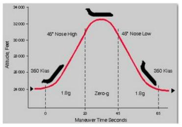
Fig 1: Course of parabolic flight (2)
