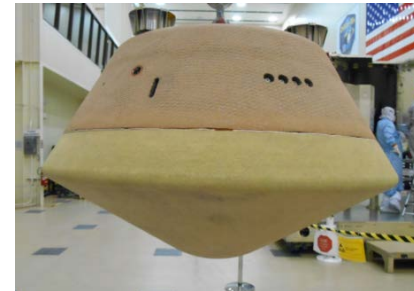
OSIRIS-REx forebody TPS. (~0.8m diameter)
