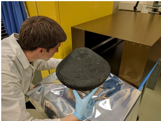
C. Partial EDU plus EDL experiment in ARCxSAT multi-use cavity (12x12x26in).
