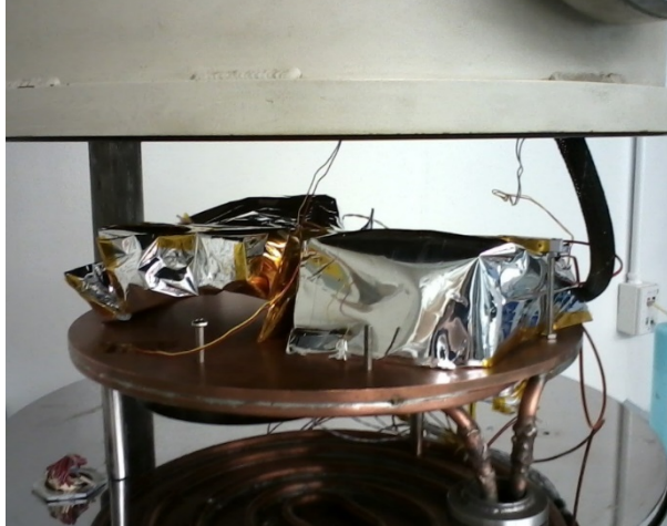
Figure 6: Thermal Vacuum Setup for 1U Heat Dissipation Test
