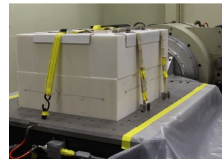
Figure 3. Foam-Mounted Flight Acceptance Vibration Test.
