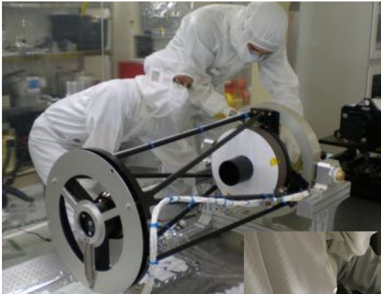
Optical adjustment work of telescope
