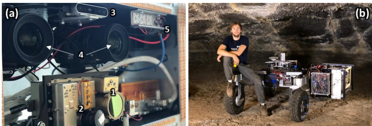
Figure 1-a. Cave instrument package consisting of point spectrometers (1), a multi-illuminant spectral imager (2), a 3D depth mapping sensor (3), stereo DSLR cameras (4), and custom photographic illumination (5). Figure 1-b. The CaveR rover used to carry the science payload and simulate a NASA planetary cave mission.
