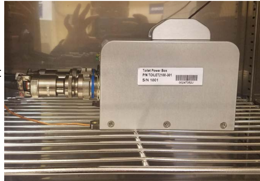
Flight Power Box in Burn-in Testing at JSC
