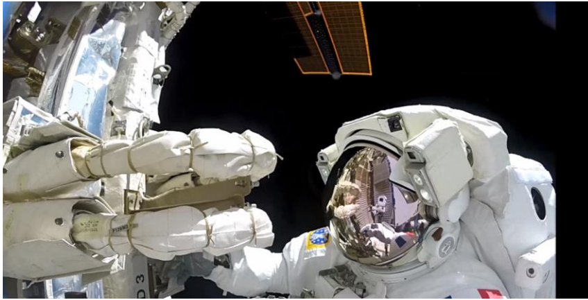
Figure 12. A screenshot from the EVA GoPro during the inspection of the P1-3-2 RBVM Supply and Return Flexible Jumpers.
