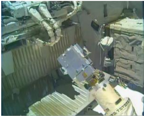
Figure 10. RELL scanning the P1-3 RBVM #2 Flexible Jumper Hose Assemblies.
