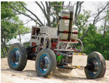
Carnegie-Mellon University / NASA Scarab Rover powered by a H_2/O_2 Fuel Cell System
