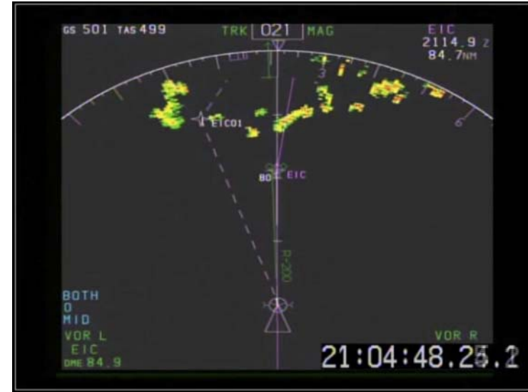
FANS-1/A CPDLC Equipped Aircraft (747-400 Navigation Display)
