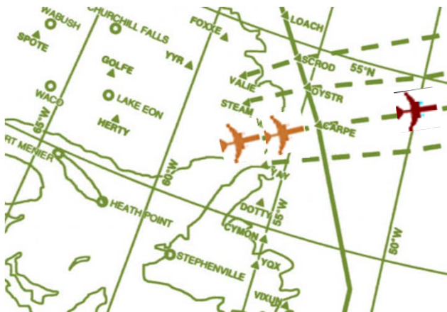
Same-Track Loading, Multiple Aircraft Interactions (Track Loading)
