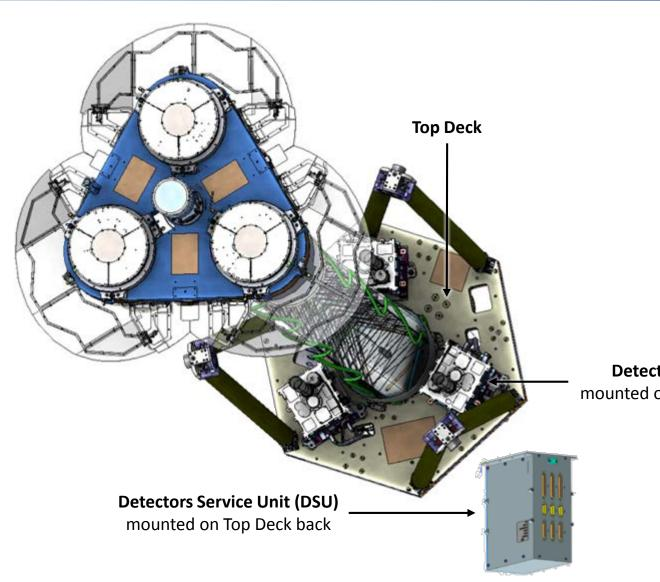
**Detector Unit (DU)** mounted on Top Deck front
