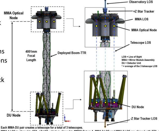
MMA 1 LOS is aligned to STA\_+Z LOS, which is aligned to MMSS Datum A. MMA 2 LOS and MMA 3 LOS are aligned with STA\_+Z LOS. Each DU is aligned to each MMA such that all 3 telescope LOS are parallel to one another and aligned with the STA\_+Z LOS.
