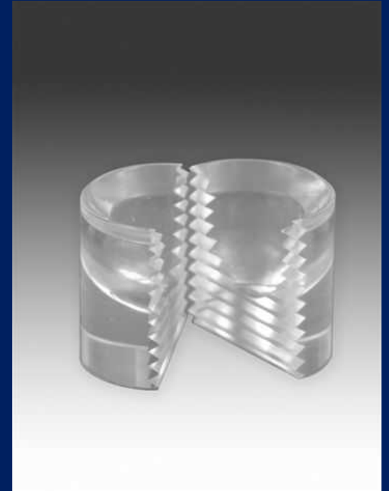
Fig 5. Polycarbonate two-piece 0.50 caliber sabot.
