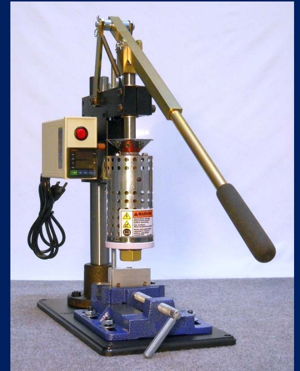
Fig 4. Injection molding Model LNS 150A. [17]
