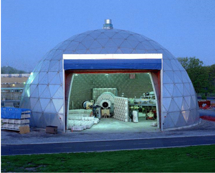
Figure 1.—Photograph of the APL laboratory. SHJAR is the smaller rig to the left of center.
