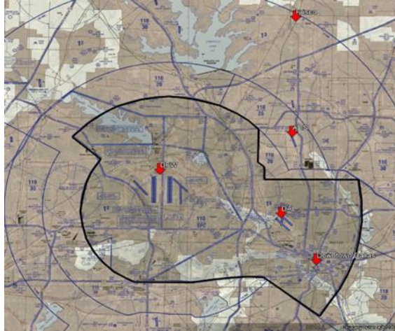
Figure 1. Class B Airspace in DFW as shown by black boundary, the red arrows show origin destination points and blue routes are helicopter routes
