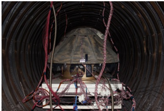
Static Pressure Test in Autoclave
