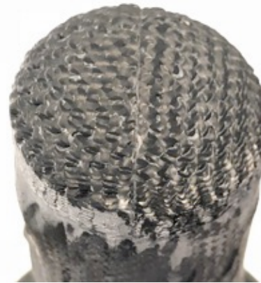
IHF 3": Hot Wall Heat Flux: 3600 W/cm 2 Pressure: 5.3 atm
