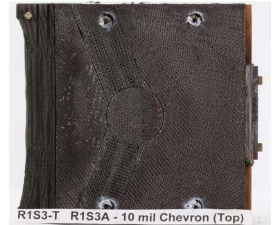
AEDC Shear Testing: Hot Wall Heat Flux: 1200 W/cm 2 Pressure: 2.9 atm Shear: ~4000Pa
