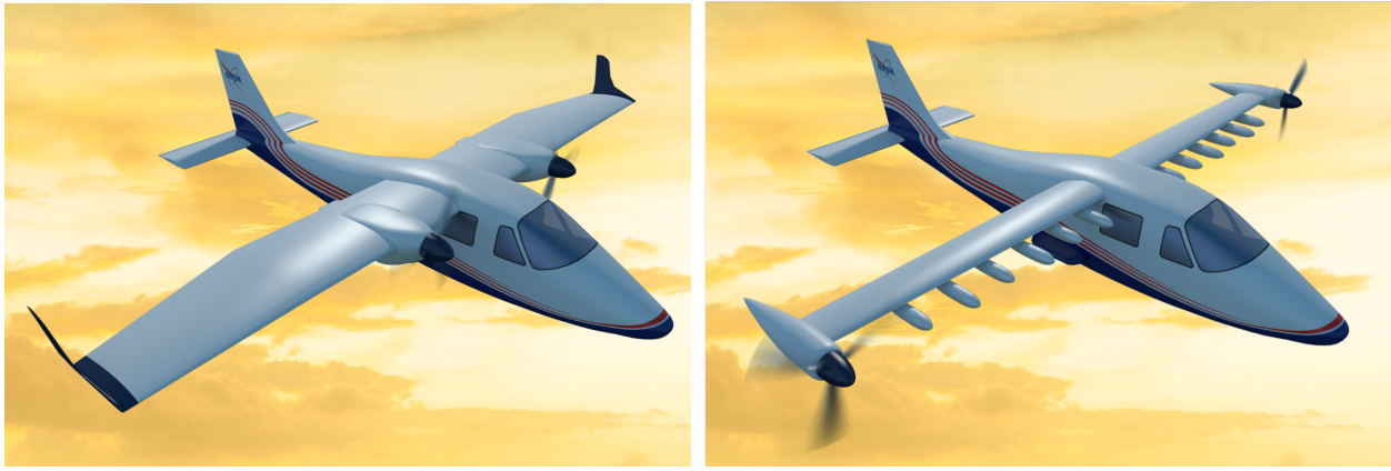
(a) X-57 Maxwell Mod II with original Tecnam wing and electric motors. (b) X-57 Maxwell Mod III with smaller wing, wingtip electric motors, and weighted high lift motor pods.
