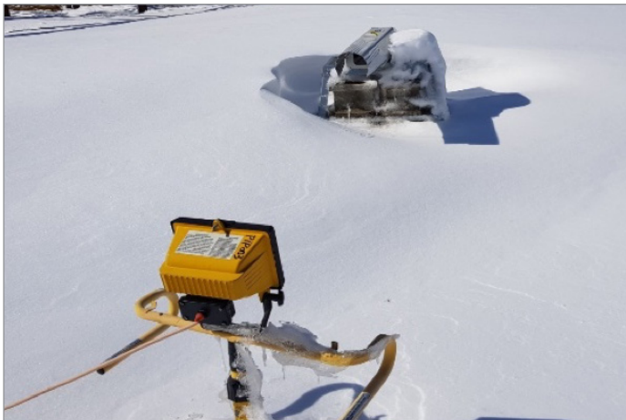
Figure 2.4.2: NASA's Precipitation Imaging Processor (PIP) in support of the 2018 Winter Olympics in Pyeongchang, South Korea. The PIP is a Wallops-built instrument that uses high resolution video to capture falling snow.
