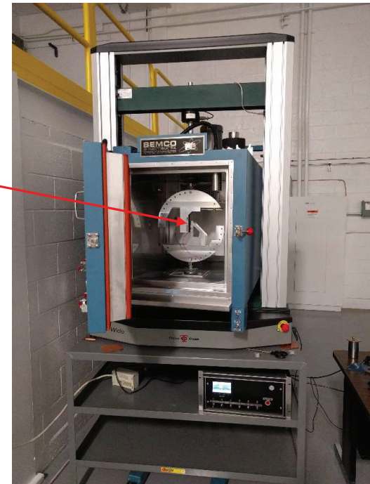
Adhesion Force Measured in environmental chamber using the newly developed NASA Glenn methodology
