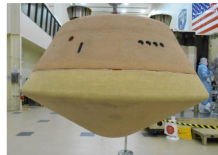
OSIRIS-REx forebody TPS. (~0.8m diameter)
