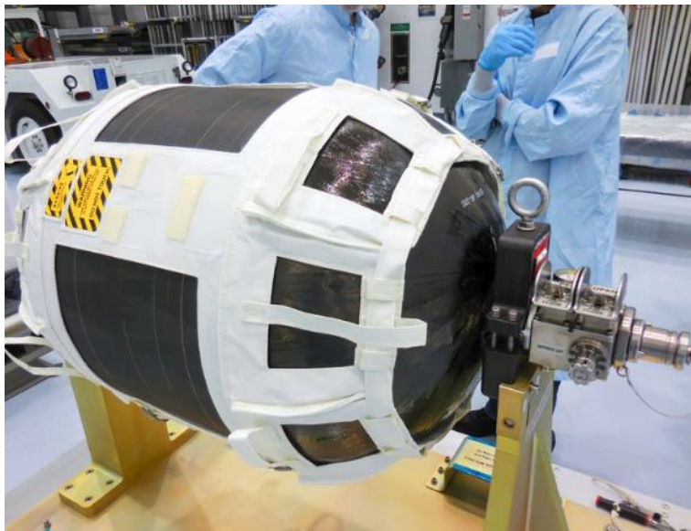
Figure 1. Nitrogen/Oxygen Recharge System Tank
