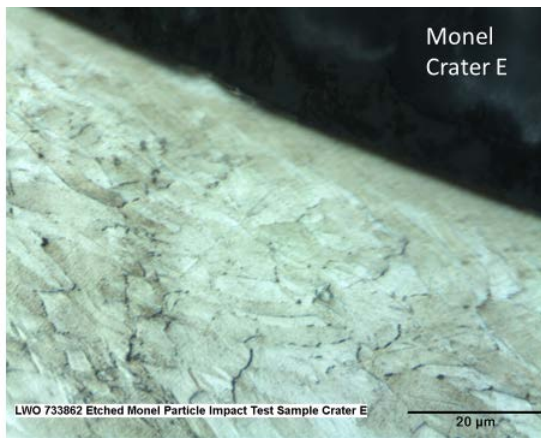
FIG. 20 – Monel 400 particle impact test target microstructure adjacent to (a)-(b) Crater E floor, (c)-(f) Crater E walls.
