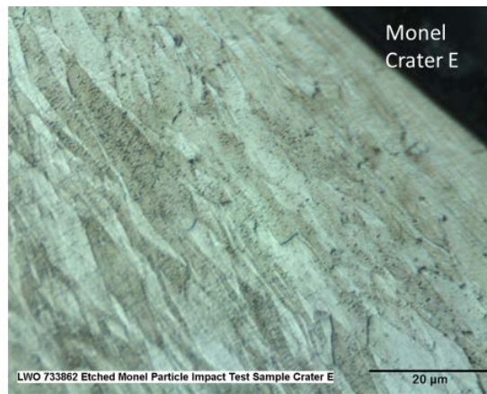
FIG. 20 – Monel 400 particle impact test target microstructure adjacent to (a)-(b) Crater E floor, (c)-(f) Crater E walls.
