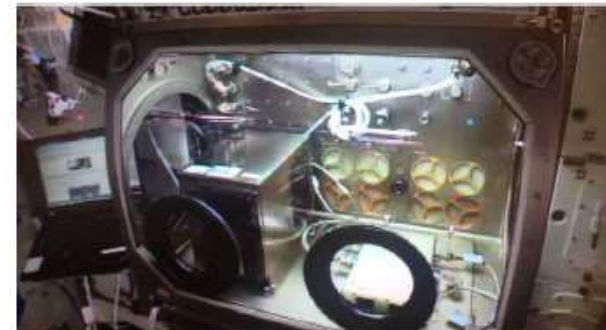
3D Printing in Zero G Tech Demo payload in the microgravity science glovebox.
