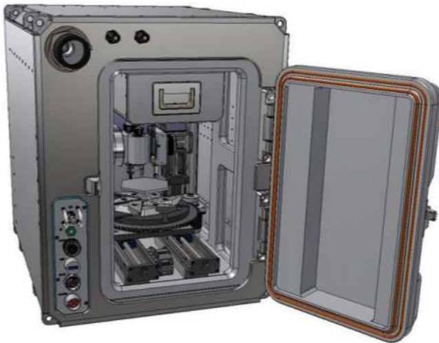
Rendering of Vulcan as a double locker ISS payload (image credit: Made in Space).
