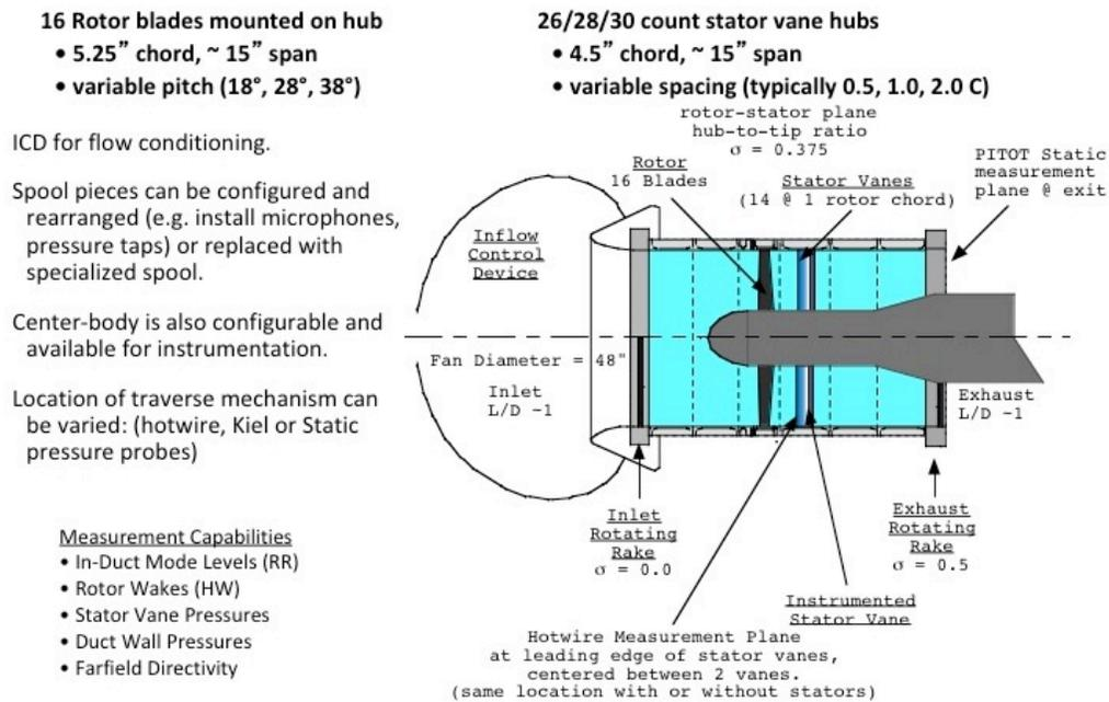
Figure 6: Schematic of ANCF Measurement Locations
