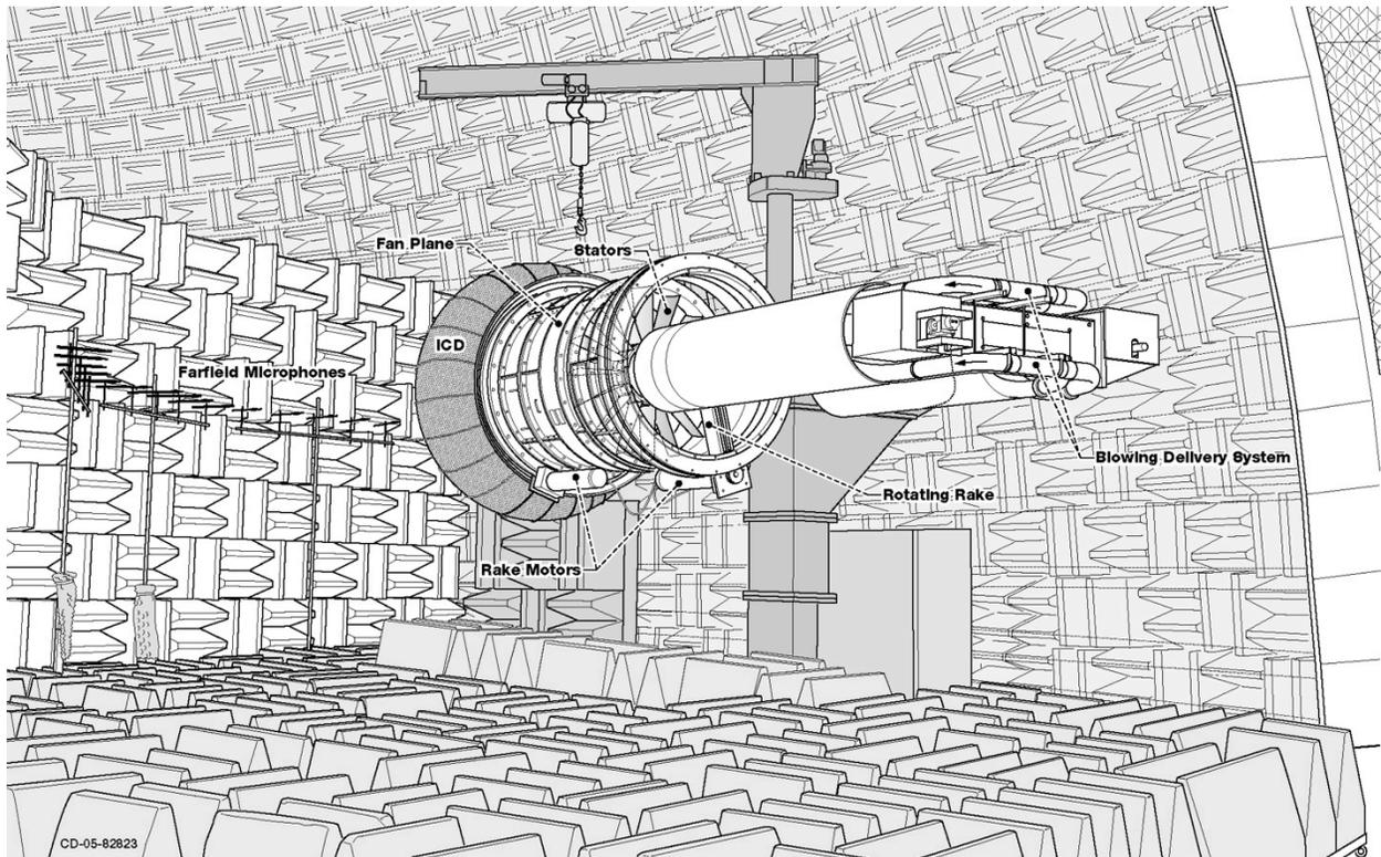
Figure A: Line Drawing of the Advanced Noise Control Fan in the Aero-Acoustic Propulsion Laboratory
