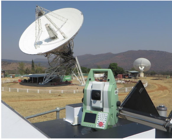
Fig. 1 The Leica MS50 Total Station of the Site Tie.
