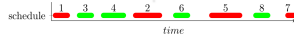
Fig. 1 Recursive scan selection. Red (dark) lines indicate observing times for main scans. Green (light) lines indicate observing times for recursively selected scans. Numbers show the order in which these scans are selected.
