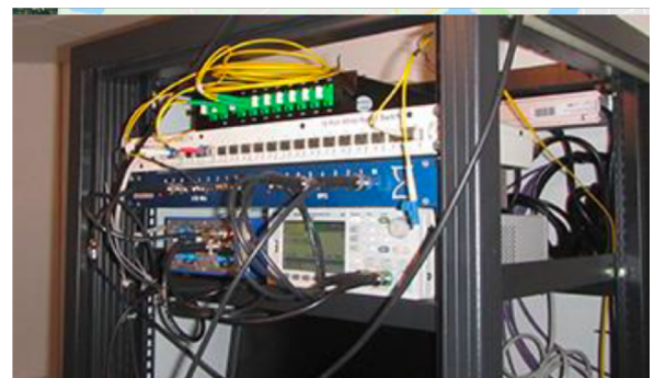
Fig. 4 Current set up arranged at Aalto Metsähovi radio observatory where the time and frequency signals provided by the VTT MIKES are being compared with the local Hydrogen masers.
