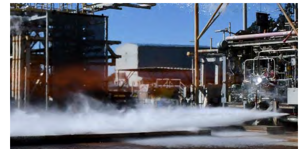
First successful hot fire test of a regen-cooled GRCop-84 3D printed MCC with an integral Electron Beam Free Form Fabrication (EBF3) deposited nickel superalloy jacket.
