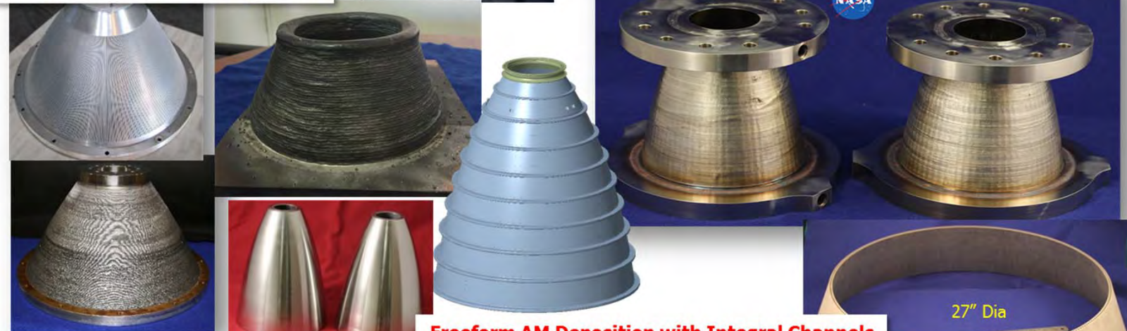
Freeform AM Deposition with Integral Channels
