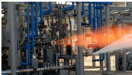
GRCop-84 AM Chamber Accumulated 6000 sec hot-fire time at full power with no issues
