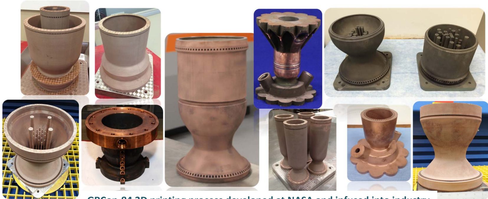
GRCop-84 3D printing process developed at NASA and infused into industry
