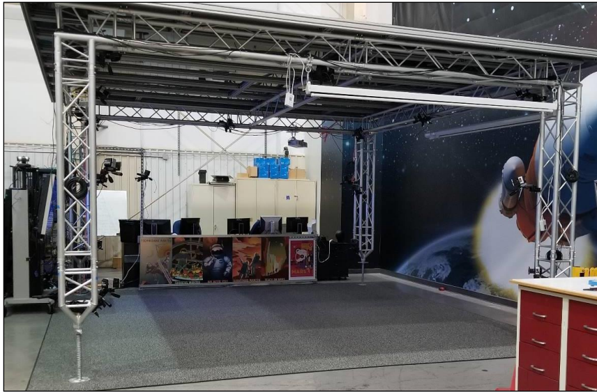
Figure 1: Virtual Environments Lab (VEL) at NASA Marshall Space Flight Center. The VEL contains a 16 infrared Vicon motion capture camera system and VR capabilities with Oculus Rift and HTC Vive.
