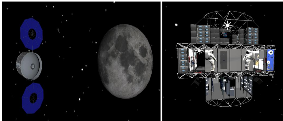
Figure 3: Outside (left) and inside (right) views of the VR mockup of the DSH. Using VR allows for more design features to be included in the VR mockup (such as the end domes and solar panels) than are feasible in the physical mockup.
