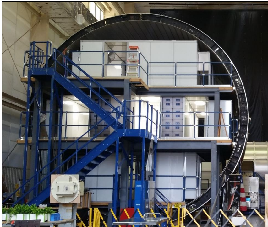
Figure 2: The physical SLS derived Deep Space Habitat (DSH) mockup. This mockup includes a galley and exercise area on the upper deck, crew quarters and laboratory equipment on the mid-deck, and a work area on the lower deck.
