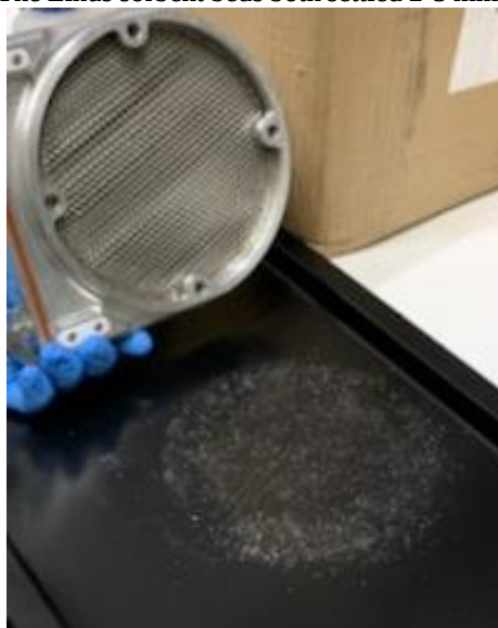
Figure 10. Dust recovered from Linus removable filters (also pictured). The black trays provide an enhanced visual contrast to view dust recovered from the filter
