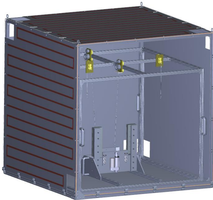
Figure 14. NEA Scout Hot Box. With One Side Removed, and Showing the Deployment Fixture
