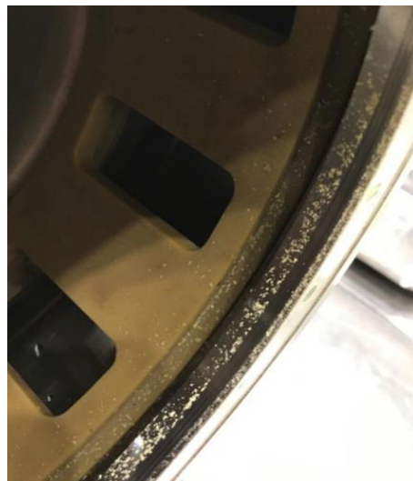
Figure 7: VariSeal shedding in centrifuge assembly after 200 hours of runtime.
