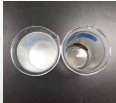
Post-Separation of 12mm fibers from ABS/Acetone solution
