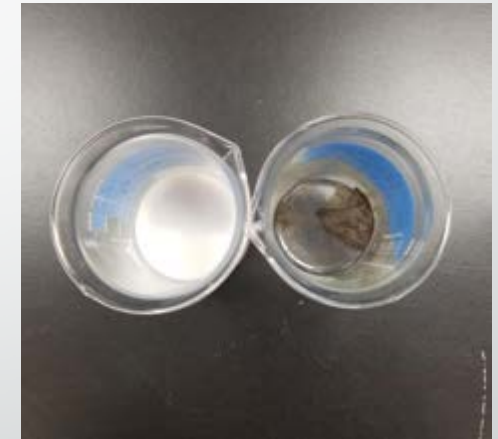
Post-Separation of 3mm fibers from ABS/Acetone solution
