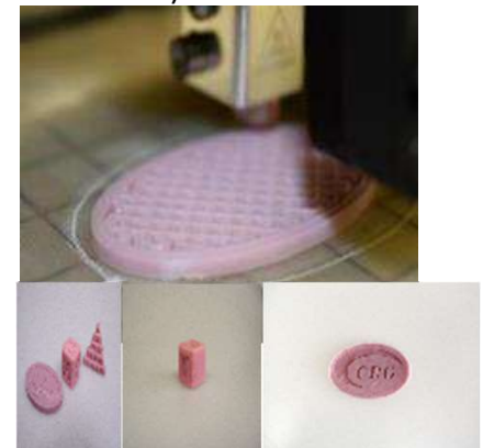
FFF prints using reclaimed anti-static bagging film with reversible cross-linking additive (image from Cornerstone Research Group)
