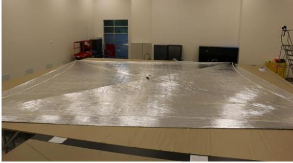
Fig. 7. Deployed NEA Scout monolithic solar sail.
