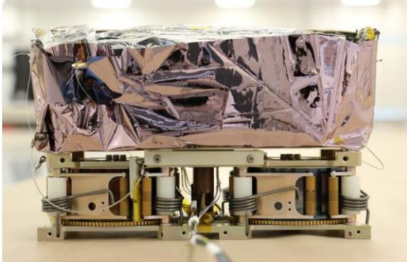
Fig. 5. As-tested solar sail deployer
