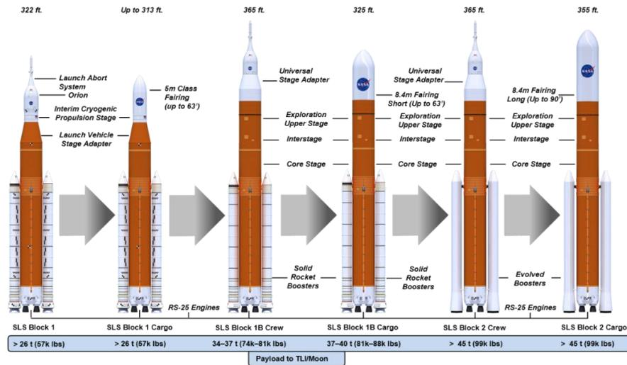
**Fig. 4: The SLS vehicle evolution path illustrating the increasing mass and volume capability.**
