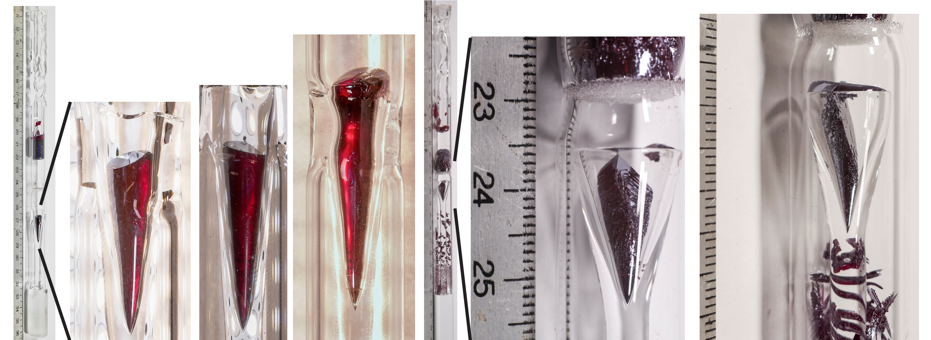
Fig. 5a: InI crystals grown in a closed setup, vacuum, and at 1.2mm/d. The crystals are backlit to show the transparency.
