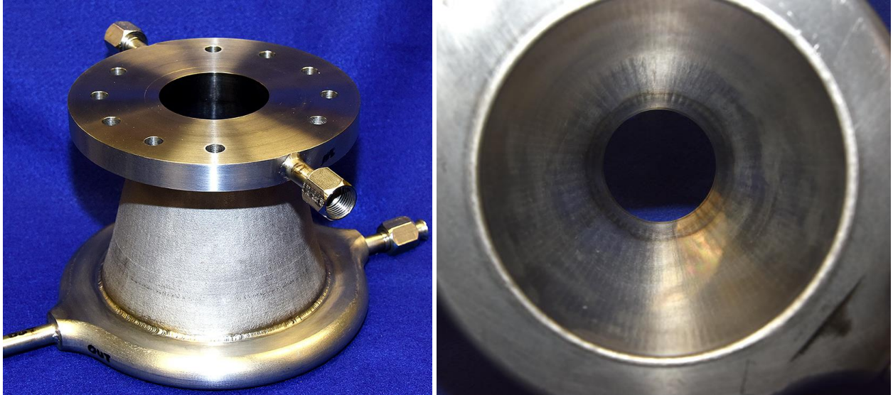
Figure 6. Completed Nozzle #3 Inconel 625: EB Welded Manifolds (left) & Final Machined Hotwall (right)
