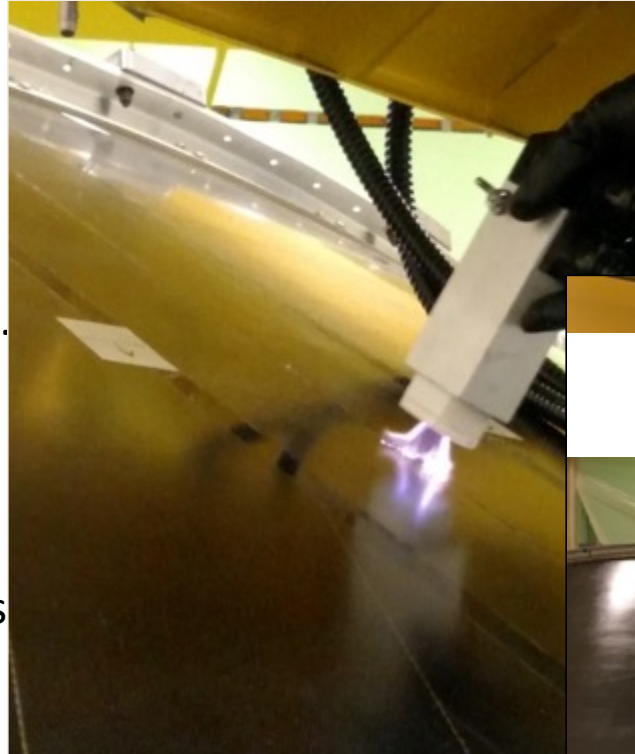
Surface Preparation with Corona Plasma Treatment
