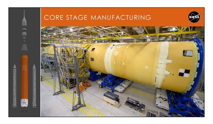
MAIN IMAGE: 4/5 of the core stage joined at MAF.
