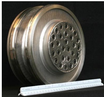
20K LPS Subscale Injector. Tested August 2013
