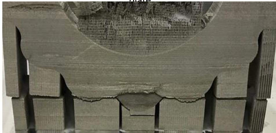
Residual stress induced failure.
