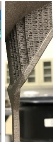
Hybrid crown & perforated block support
