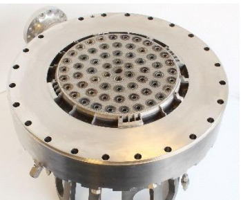
35K AMDE Injector with Welded Manifolds, Tested 2015
