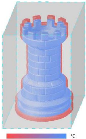
Cooling shrinkage behavior.
