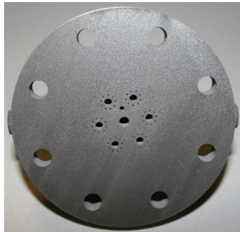
100lbf LOX/Propane Nanolaunch Injector. Built 2012. Tested 2013.
