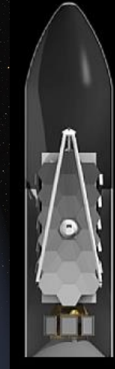
8.4m Fairing with Large Aperture Telescope
