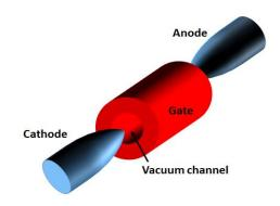
Vacuum provides the fastest electron speed, better than any semiconductor. Nevertheless vacuum tubes were bulky, fragile and consumed much power. Now nanotechnology has enabled fabrication of vacuum tubes at nanoscale in silicon chips. The speed, immunity to radiation and high temperature operation are expected to revolutionize space electronics.
