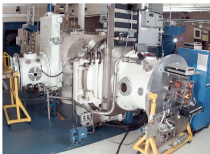
NASA GRC VF-8 Low-Power EP Test Chamber
