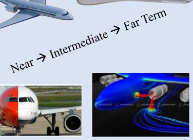
Acoustics, operability and aeromechanics challenges have arisen for turbofans as the pursuit of higher propulsive efficiency has pushed engine configurations and installations outside of the existing experience base. Near term research will inform integration of the next generation engine with the wing and provide learning for far term configurations.
