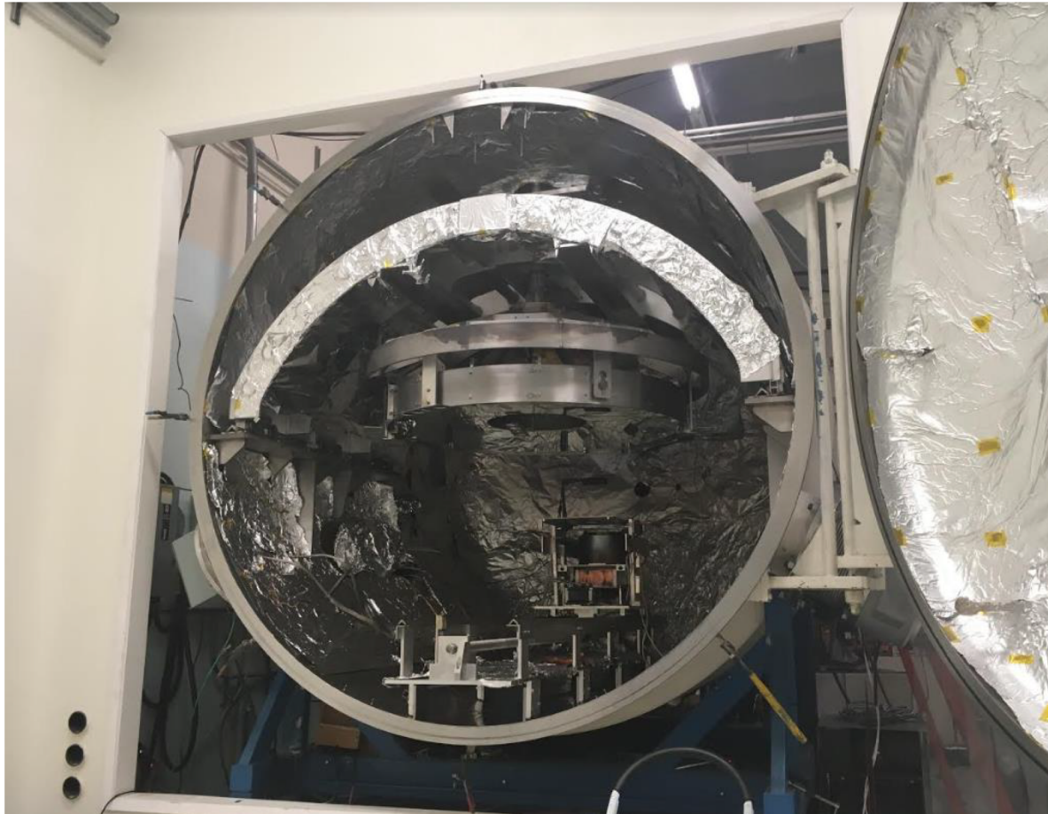
ZeCoat's 2.4-m diameter coating chamber with a 1.3-m diameter 900-lb mirror after silver coating
