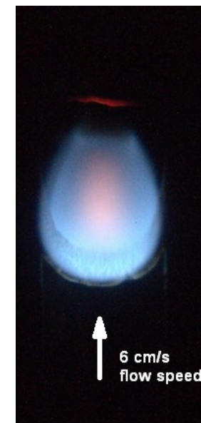
Flame burning PMMA slab in \mu g from BASS experiments.
