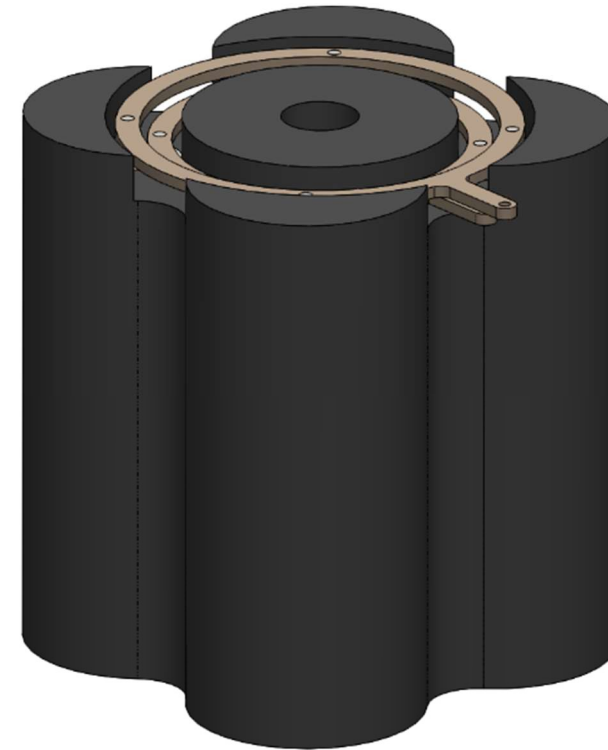
Electrical Heat Source simulates 8 x LWRHU
