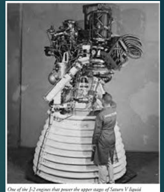
One of the J-2 engines that power the upper stages of Saturn V liquid
