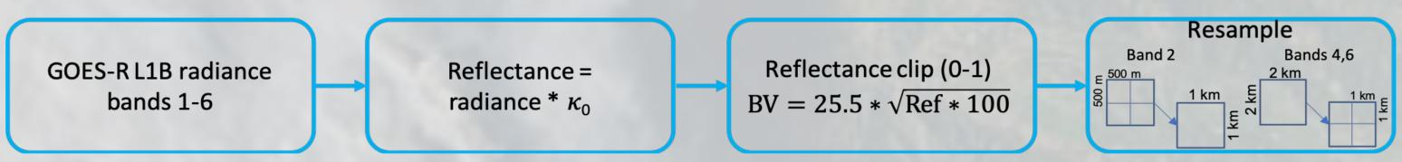
Training data developed by manually labeling boundaries of smoke in GOES 16 imagery. For training the model, GOES L1B radiance data is downloaded from NOAA-AWS repository. Radiance values are then converted to reflectance and bands 2, 4 and 6 are resampled to 1 km pixels.
