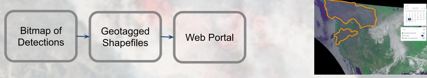
Model predicts the probability (p) that a pixel is smoke. A bitmap of the predictions (p > 0.5) are then geotagged and converted to shapefiles. These files are rendered and visualized in an online web portal for each day, and is also available through an API in GeoJSON format.
