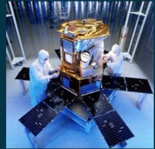
SORCE is 290 kg based on an Orbital LEOStar-2 bus
